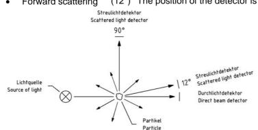
As shown in the figure above, an intense collimated beam of light is projected through a sample contained within the sensor. The intensity of this light beam is measured by the direct beam detector, located opposite to the light source.
