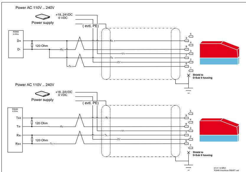
The 120 Ohm resistors are not built into the device. They must be provided externally and are absolutely essential for the RS485 current loop operation.
