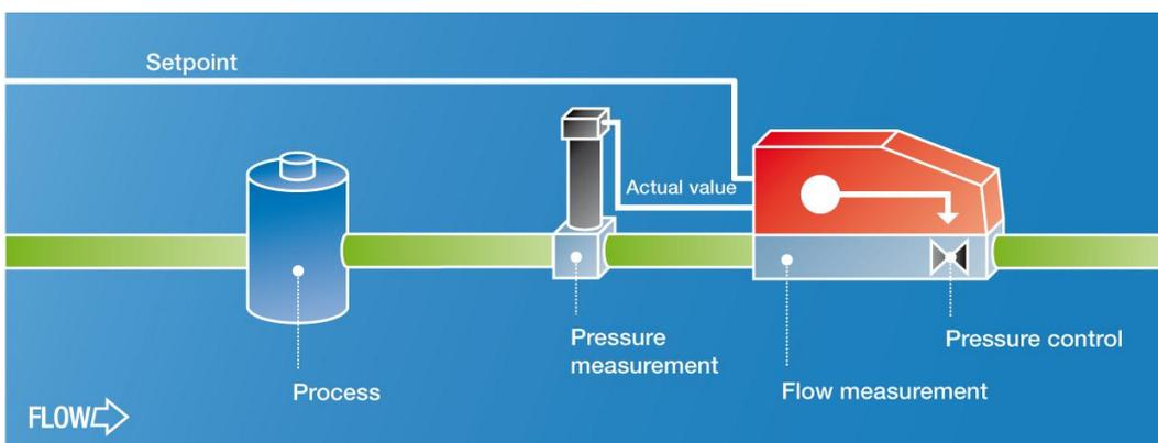
The pressure at the outlet of the pressure controller is lower than the pressure in the process i.e. the pressure that is to be controlled.
