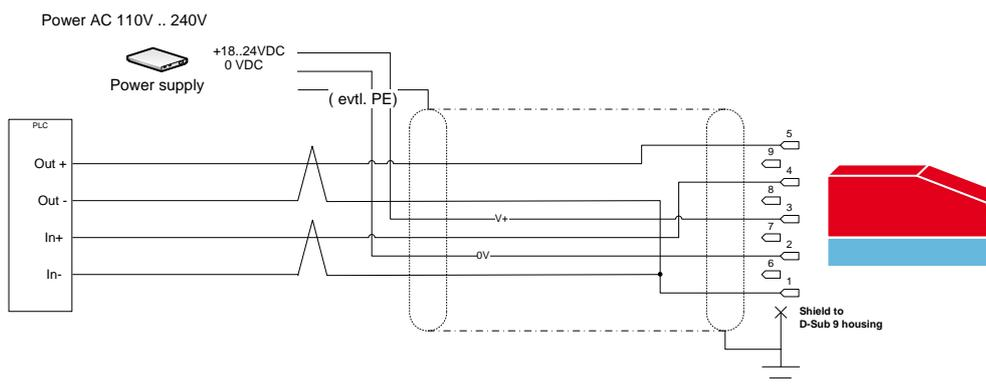
For precise measurements we advise against combining the 0V-supply and comm wires. Please run the cable as shown above in the illustration.
