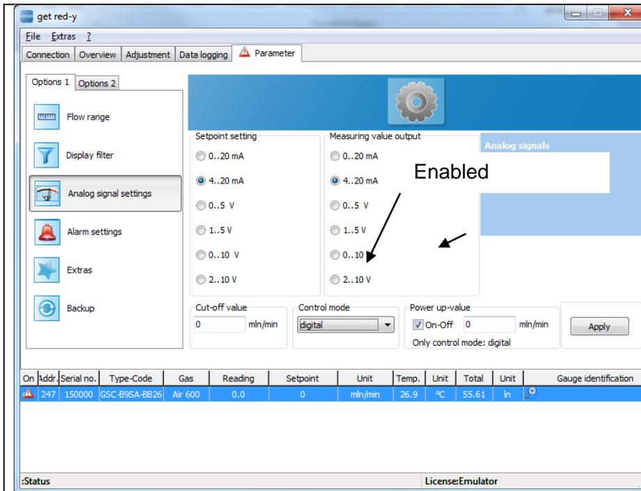
When the device is in digital **control mode** and the **Startup-Set point** is switched on.
