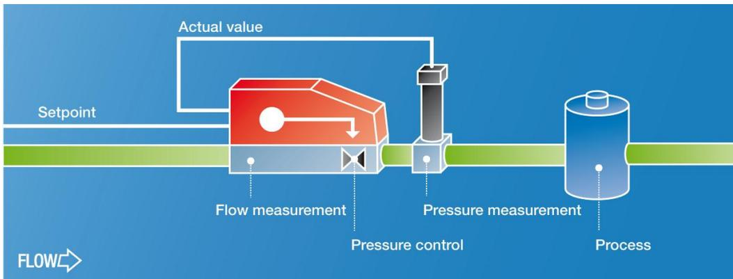
The pressure at the inlet of the pressure controller is higher than the pressure in the process i.e. the pressure that is to be controlled.
