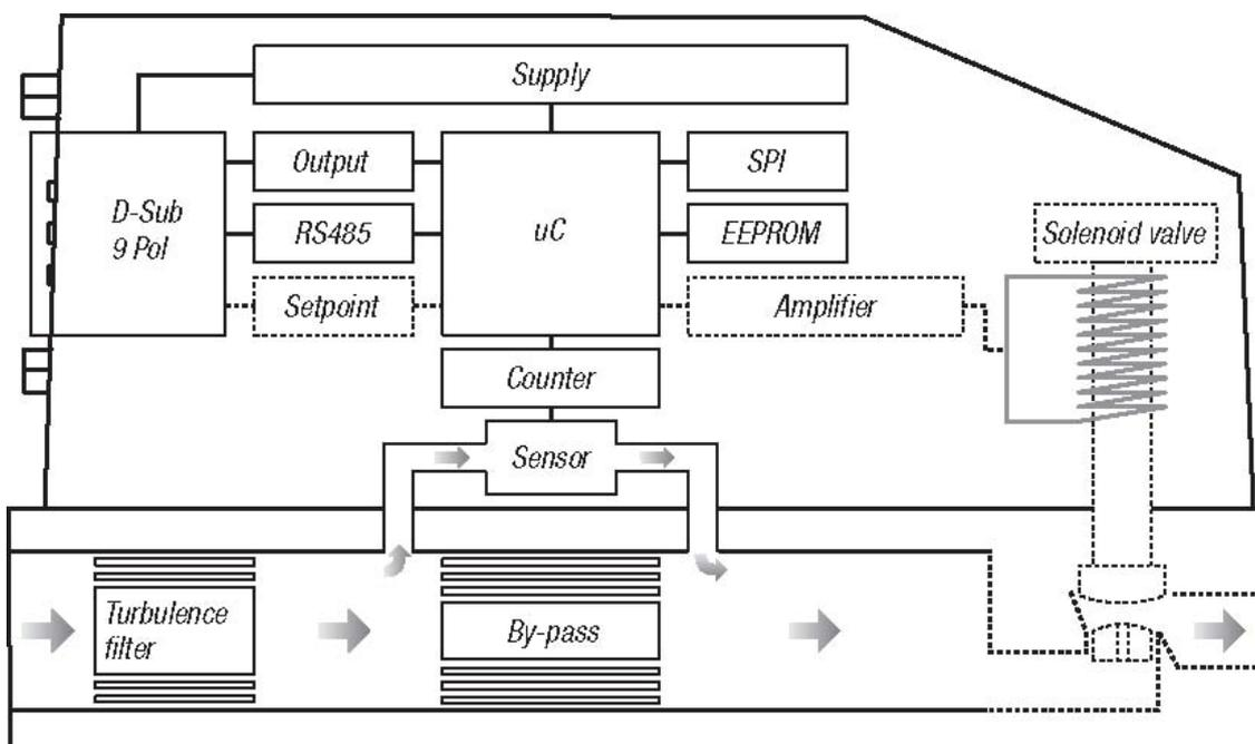
Figure 3: Block diagram
