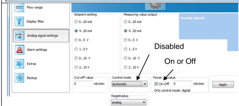
If the device is in automatic or analog control mode the display of the flashing LED will be suppressed.
